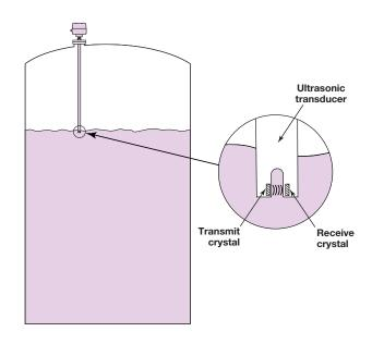
Ultrasonic signal transmission across transducer gap
